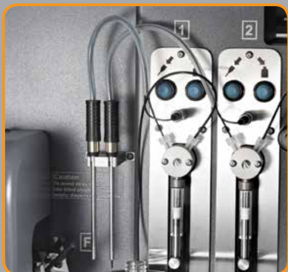
Figure 1 Reagent dispensers allow for easy and accurate reagent addition.
